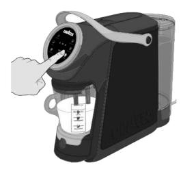
8 When ready, the machine will deliver the measure of coffee in the jug and will automatically stop.
