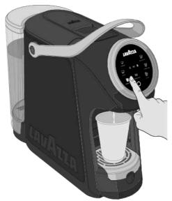
To increase the effect of the descaling product, the machine will automatically pause a long time.
