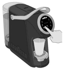
Open and close the lever, remove and empty the cup, then supply water one more time by pressing the coffee selection.
