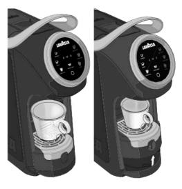
Position the cup or mug on the cup rest grid, then pull up the capsule loading handle.
