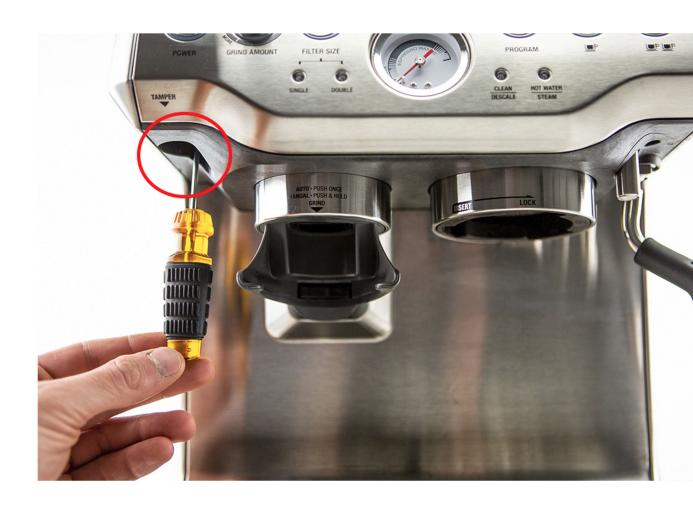
Locate and remove the screw located directly in Front of the steam wand and water spout.
