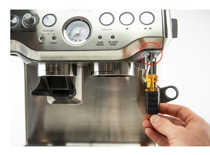
Remove the water tank from the back of the machine and use a philips head screwdriver to remove the five screws found at the top of the back panel.
