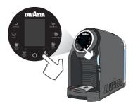
Press System Clean button and follow  $(\Delta)$ steps shown on machine display.
