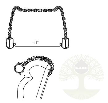
Wrap the speakers around the chair's headrest with the volume knob on the left for the user at about ear height.
