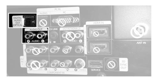
On the back or side of your TV, find the DIGITAL AUDIO OUT (OPTICAL) port. If audio out ports are not available on your television, use the audio ports on your cable or satellite box.
