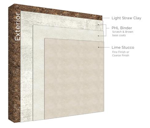
• Specialized plaster formulas made with high plasticity lime and pumice pozzolan for excellent workability, adhesion, and durability.
