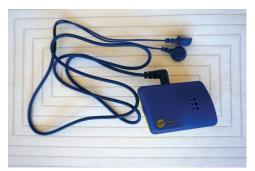
Sensor mats require the urine to penetrate through the underwear and usually a bedsheet, making it less sensitive to minor accidents.
