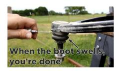
4: If you hear the bushing squeak, you need to add grease. When adding grease to the bushing, be aware that excessive pressure can cause irreversible deformation of the polyurethane bushing. The picture shows the deformed and failed polyurethane bushing.
