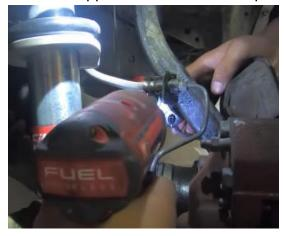
4.Remove the cotter pin from the upper ball joint. Take off the castle nut from the top of the upper control arms.
