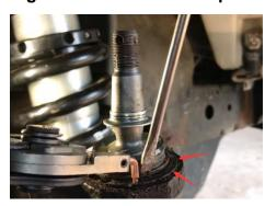
8. Remove the original upper control arm and replace it with a new arm.
