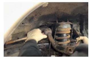
7. Remove the ball joint from the the knuckle.
