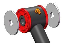
NOTE: Make sure that a washer is placed on each side of the bushings. Then, carefully
