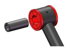
3. Pay attention to the position of the zerk fitting. After installing the kit, screw on the zerk fitting and use a Lever-Action Manual Grease Gun to lubricate it.
