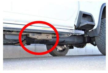
3. Assemble the main body of the Traction Bar.
