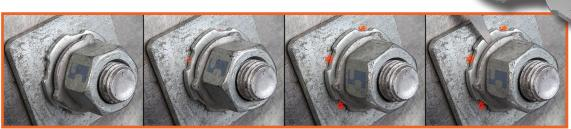
SQUIRTER® DTIs (Direct Tension Indicators) are DTIs with flexible silicone embedded in the depressions under the bumps. To use them, simply tighten the bolt until the calibrated amount of orange silicone appears from under the DTIs squirt locations, then stop tightening. That's all there is to it.
