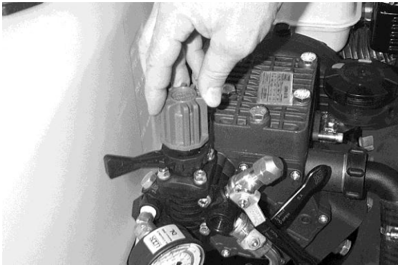
Photo 13 Kappa 43 Pressure Adjustment
