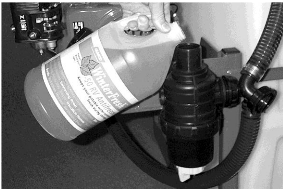
Photo 23 Add Anti-Freeze through Suction Strainer
