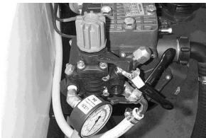
Photo 9 Kappa 43 Pressure Regulator Bypass Position
