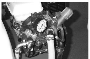
Photo 11 Kappa 40/55/75 Pressure Regulator Bypass Position
