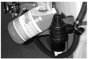
Photo 23 Add Anti-Freeze through Suction Strainer
