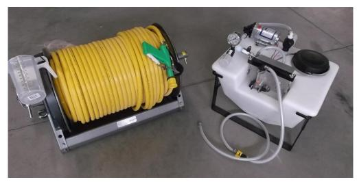
Pulling the primary trigger of the dual trigger gun causes the fertilizer solution to spray out of the discharge nozzle. The Eco-505 injects pesticide solution into the flow of fertilizer at the gun, just before the nozzle, by pulling the injection trigger on the gun while holding down the primary trigger.
