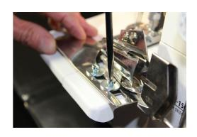
Cut binding tape to a angle / point and feed tape into the binder.
