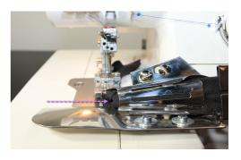
Once your binding task is complete, remove the binder attachment from bracket using the M4 slotted screws with flat screw driver.
