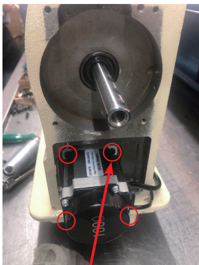
步進電機固定螺絲 X4 Stepper motor stabilized screw *4
