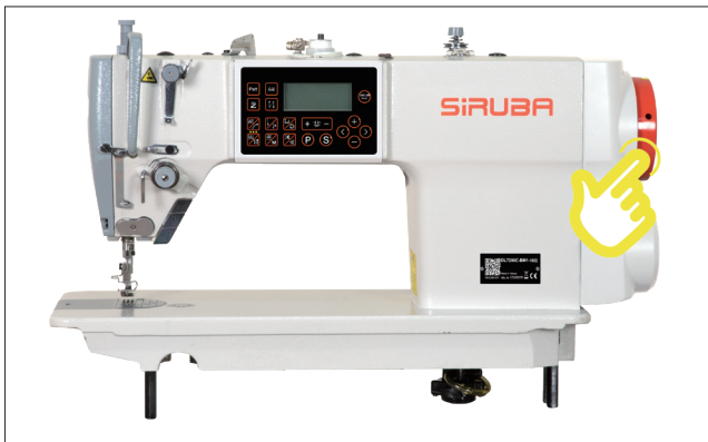
手動轉動手輪至上停針位 Spin the handle to top needle stopped point
