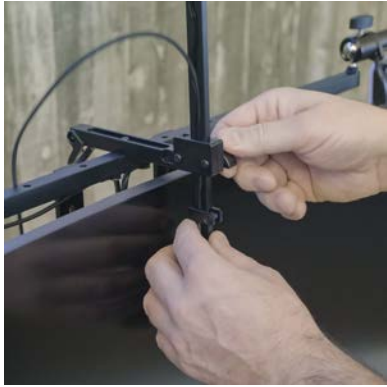
Adjust the friction on the Camera Bar slide with the front Thumbscrew
