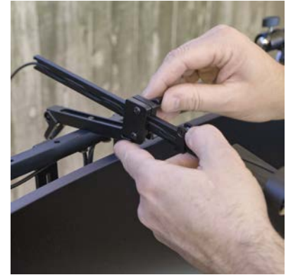
Adjust the friction on the Camera Bar pivot with the screw on the mount
