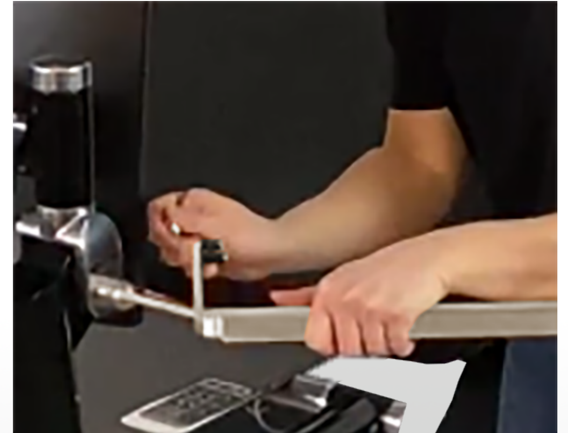
STEP 3: Use the hex key to tighten the screw. Wiggle the laptop mount back and forth as you do this to make sure it is tight. Even when the screw is tight, the mount will still move a little in the lug.
