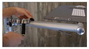
Install C-shaped mount over the small section of the desk arm
