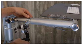
Slide C-shaped mount onto the larger section
