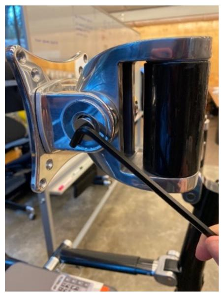
Use the wrench to tighten the screw as required. Be sure to insert the wrench fully into the socket in the bolt head so the interface will not be damaged if you need to apply a lot of torque. you can adjust the tension so the pivot will not normally slip but you can still adjust he monitor manually if you need to.
