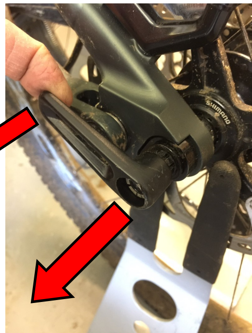
Figure 20: 12mm QR Axle Re-Positioning Lever Arm
