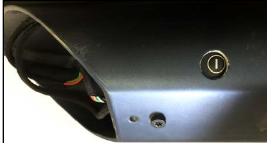
Figure 56: Bosch Battery: Location of On/Off Button with Battery Fitted into Down Tube
