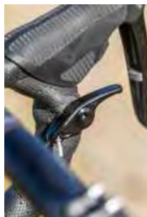
The Friston's kinked seatstays and its handlebar-mounted remote control for the dropper seatpost
