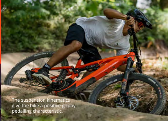
The E-160 layout is familiar but the mainframe is all new for increased stiffness, and easier, bigger battery management.
