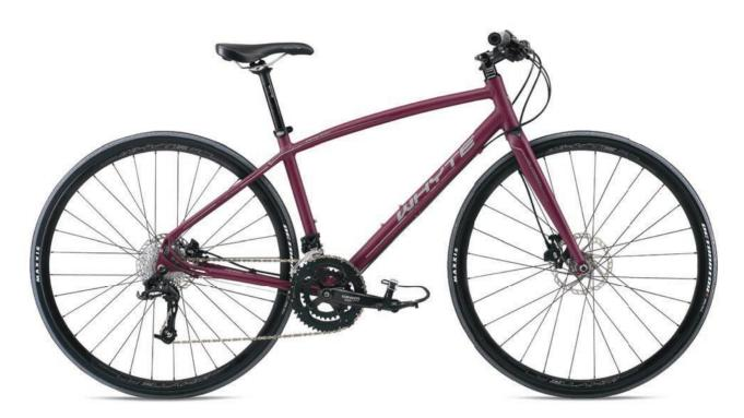
Based on our high performance mountain bike geometry, the Pimlico has a long wheelbase and relaxed head angle for high speed stability, a shorter stem for excellent slow speed manoeuvrability and slightly shorter and lower top tube to fit a woman's physique better.
