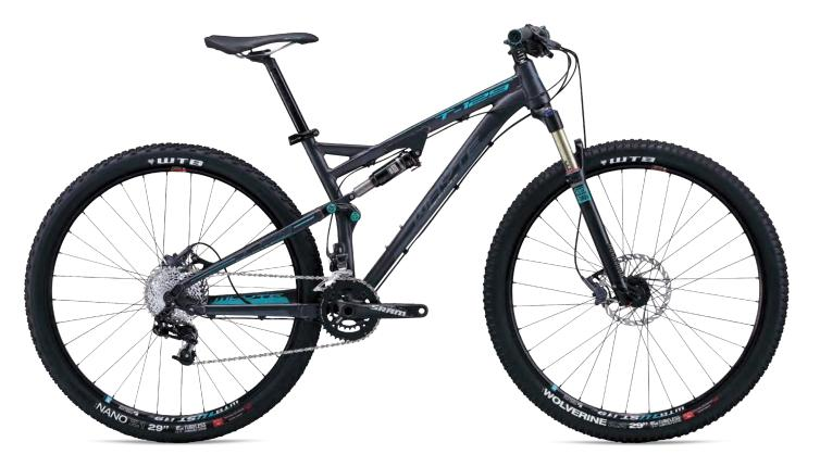
Our new Quad 4 suspension layout allows us to apply our contemporary 29er Trail hardtail geometry to the 120mm Suspension Tail Bike category. Short chainstays gives this bike the agility of a 26" wheel bike but with the inertia and terrain "flattening" advantages of a larger 29er wheel
