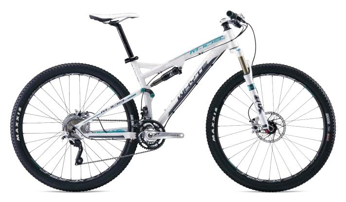
Conceived as the ideal Marathon/Endurance ride, our 100mm travel M-109 bikes are designed for long, high-speed days in the saddle. Our Quad 4 suspension layout creates room for a larger 29" wheel and is built around lifetime bearings for smooth operation today and forever quaranteed
