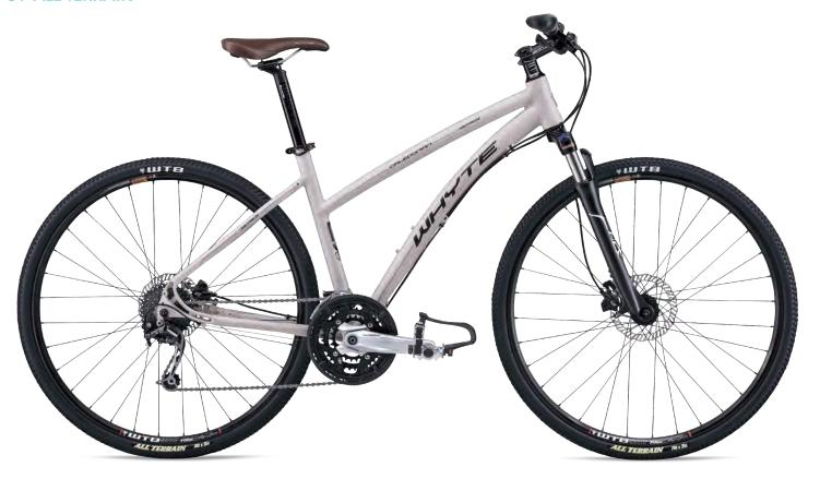
All the same key design features as the men's version, with the added benefit of a partially dropped top tube. This increases standover height, while still keeping enough room inside the frame to comfortably fit a water bottle
