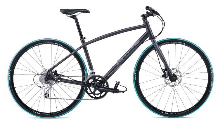
Based on our high performance mountain bike geometry, the Victoria has a long wheelbase and relaxed head angle for high speed stability, a shorter stem for excellent slow speed manoeuvrability and slightly shorter and lower top tube to fit a women's physique better
