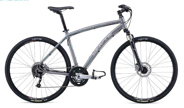
Our custom built frames are loaded with unique design touches and British weatherproof features - such as the forward facing seat slot that stops water spray from the rear wheel getting into the frame and the continuous outer cables that keep the gear shifting working smoother for longer
