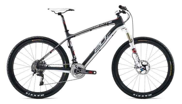
The 20-C Team bike is specced using the FSA SLK Carbon PressFit 30 crankset combined with XTR brakes, XTR drive train, and the all new Easton EC70 full uni-directional carbon wheels
