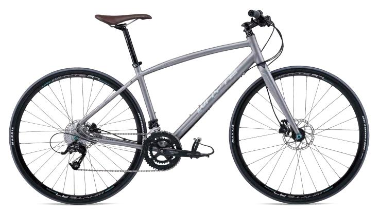
Based on our high performance mountain bike geometry, all our Fast Urban bikes have a long wheelbase and relaxed head angle for high speed stability, and a shorter stem for excellent slow speed maneuverability
