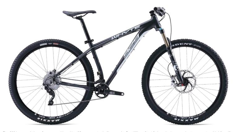
The 929 is an evolution of our ground breaking 29er geometry, built around a Fox 120mm front fork and using very short rear centre, this bike will bring "flow" to your riding, as well as the other advantages of the bigger wheels
