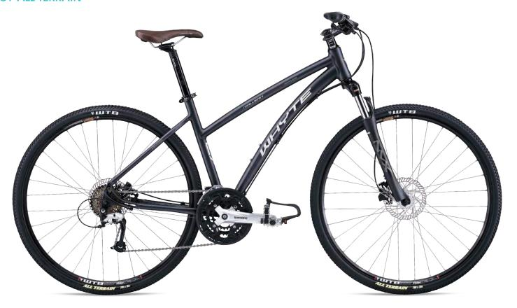
All the same key design features as the men's version, with the added benefit of a partially dropped top tube. This increases standover height, while still keeping enough room inside the frame to comfortably fit a water bottle
