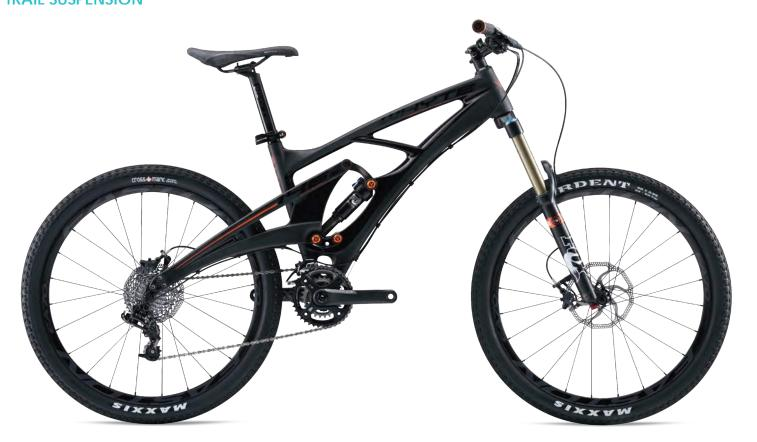
The 146 S is built around exactly the same ground-breaking full carbon monocoque chassis and swingarm as the Works and XI models. For 2013 it now features the same lightweight finish as the XI model.
