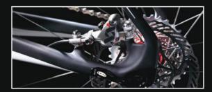
By mounting the caliper inside the rear stays with our unique dropout, we can feed the brake loads into the chainstay, allowing us to use much less material in the seat stays. This improves comfort and saves weight.
