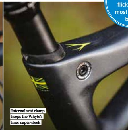
Internal seat clamp keeps the Whyte's lines super-sleek
