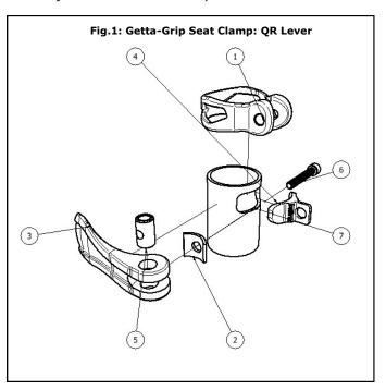
To Adjust the seat height with the QR Lever assembly fitted, simply undo the QR Lever (3) from the Closed position to the Open position. Next adjust the height of the Seat Post to the desired level, and close the QR lever (3) from the Open position to the Closed position. The QR closing force can be adjusted and optimised by turning the QR M5 Adjuster Bolt (6) clockwise or anti-clockwise with the use of a 4mm allen key before closing the QR Lever (3).
