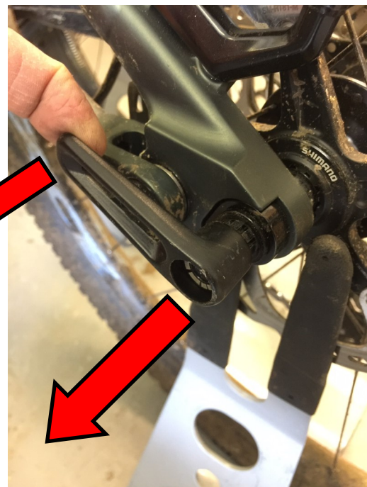
Figure 20: 12mm QR Axle Re-Positioning Lever Arm
