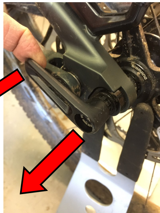
Figure 11: 12mm QR Axle Re-Positioning Lever Arm
