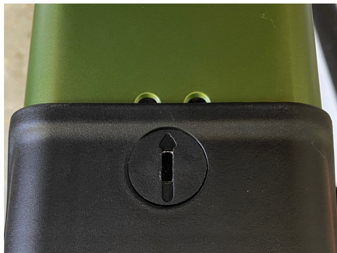
Figure 5: Position of the slot indicating the Cover can not be removed.
