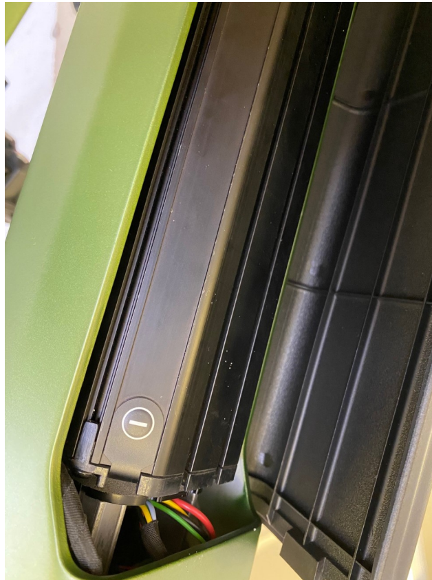
Figure 6: Bosch Battery: Location of Bosch Power- Tube On/Off Button with Battery Fitted into Down Tube and Down Tube Bat- teryCover removed.
