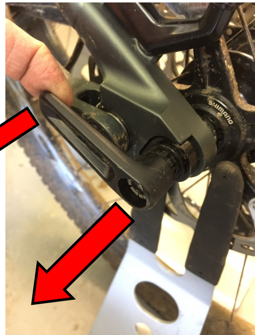
Figure 2: 12mm QR Axle Re-Positioning Lever Arm
