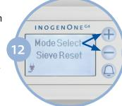
Press and hold the plus (+) and (-) minus buttons for 5 seconds. The screen will display "sieve reset" message. Release buttons once message is displayed on screen.
