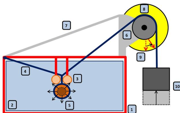
**Fig. 1** Schematic drawing of an apparatus for measuring swelling against constant force. 1—Base made from Merkur blocks, 2—crystallizing dish with isotonic solution, 3—two polyamide rollers, 4—textile strap, 5—dilator, 6—pulley, 7—arm fixing the pulley, 8—protractor, 9—pointer, 10—weight
