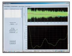
The Advanced Driveline Vibration Analyzer includes order tracking, which allows the user to monitor a particular vibration order over the cursor-defined area in order to pinpoint vibrations. This data can be correlated to speed to determine the relationship between speed and vibration.
