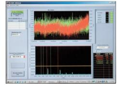
The Advanced Driveline Vibration Analyzer's sensor graphs are colorkeyed to match the analysis graph so users can quickly identify which signal is being analyzed; color-coded cursors that line up with typical vibration sources are also included. Both linear and torsional vibration information can be reviewed to quickly pinpoint the vibration issue.
