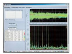
In Linear or Torsional Analysis mode, the "autoplay" feature allows users to playback the data as if the vehicle is in motion. The cursors on the signal graph can be moved to select a particular data area to analyze – there's no need to review the entire file! Data detail can also be easily viewed with the software's "pan", "zoom" and "scale" functions.
