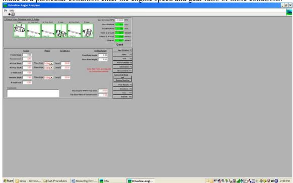
On the upper right, the calculated torsional vibration due to u-joint excitation will be displayed. In the Corrective Mode, changes to the axle angles and drive shaft angles can be made and the resulting torsional vibration measured.
