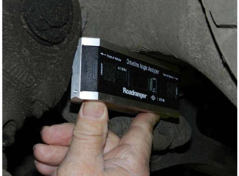
Next measure the interaxle drive shaft. A v-block is available to assure that the
