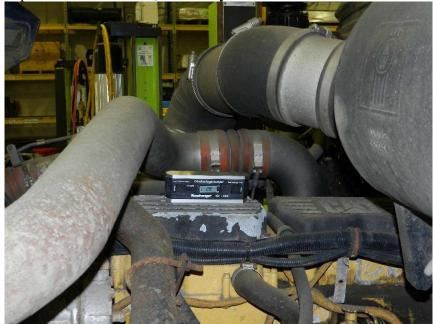
Next, measure the angles of the various main drive shafts. Make as many measurements as there are drive shaft segments. These measurements may be made at the top or the bottom of the shaft. Heed the direction of the arrows "Front of Vehicle "and "Rear of Vehicle". Note also the arrow pointing down at the left of the LED. This reading is a positive 0.9 degree angle with a downward slope toward the rear of the vehicle. (See
