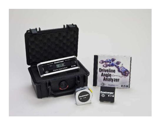
Improper driveline angles can be the source of uncomfortable and destructive torsional vibration. Being able to measure these angles correctly is the first step in diagnosing a problem and ultimately taking corrective action.
