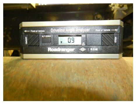
Next, measure the front axle on the arm of the axle near the spring mounts. This
