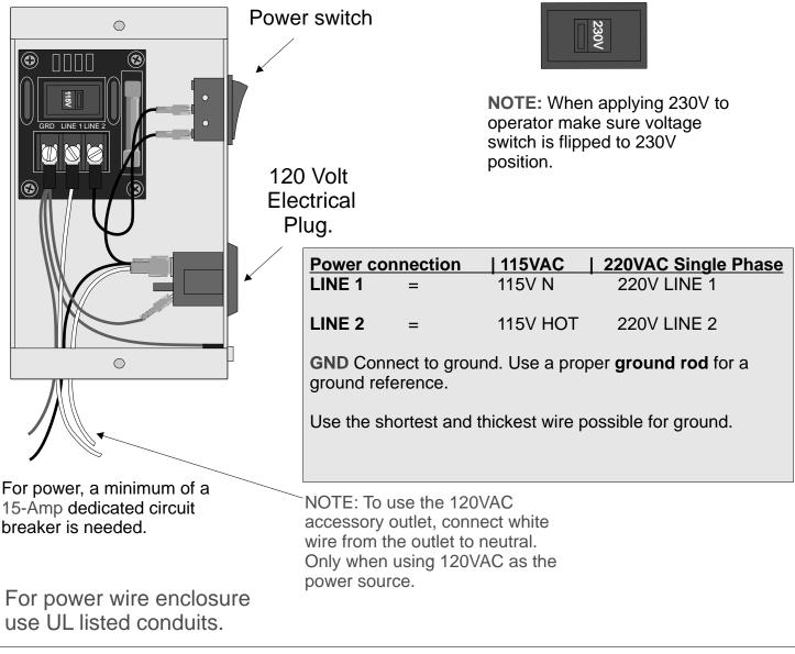
All gate operators MUST be properly grounded.
