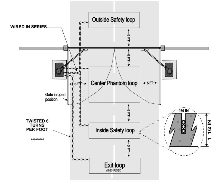
This is a normal loop layout. Remember when connecting to an All-O-Matic circuit board you use the **normally closed contacts** from your safety loop detector and **normally open contacts** from the exit loop. You must twist your wires from your exit point of the saw cut all the way to the circuit board, no exceptions.
