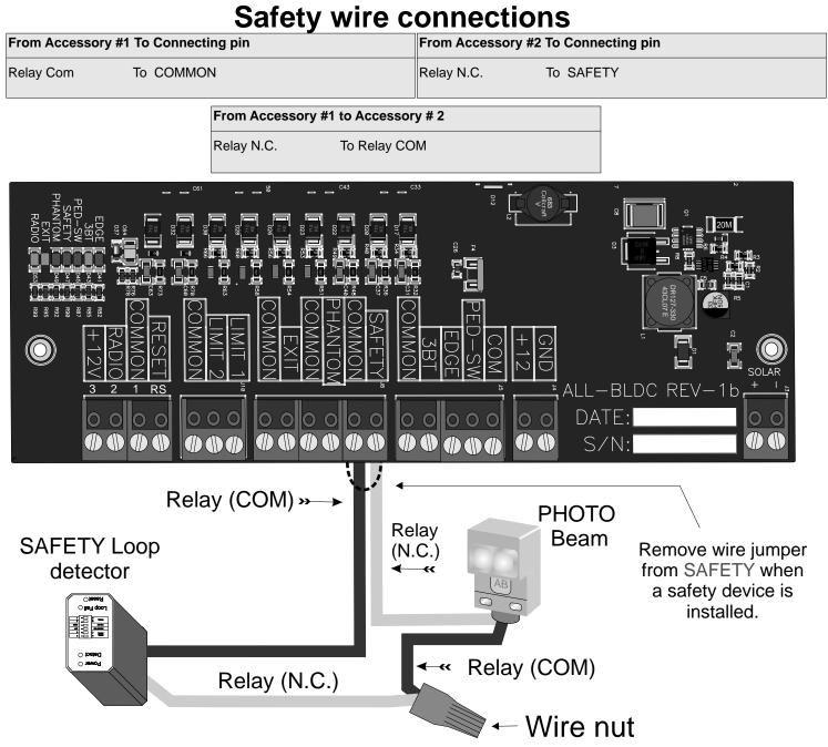
This diagram is for the relay wires of the safety devices, two wires to the board connections (one from each device) and two wires to the orange wire nut.
