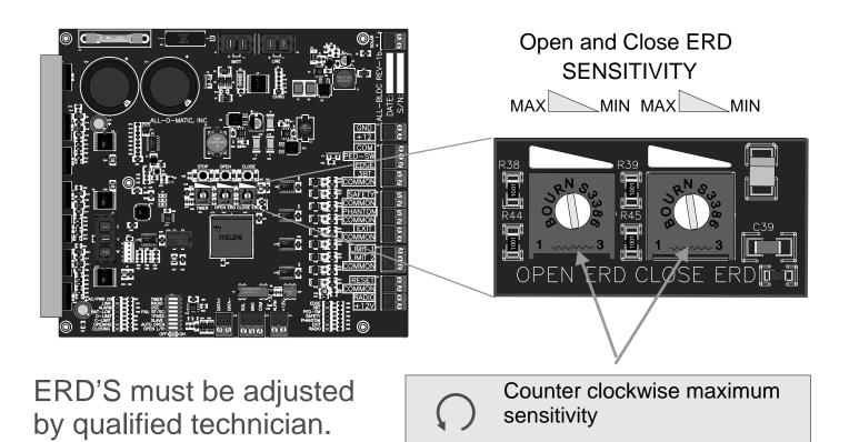
The gate operator ERDs must be adjusted so that the gate provides regular, reliable and safe cycles.
