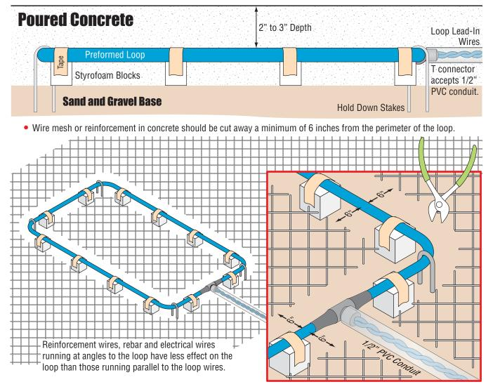
• If installed with asphalt pavement, cover the loop with 1-inch minimum of soil or sand to protect the loop from hot asphalt.
