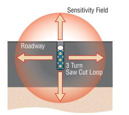
**Cutaway of Underground Loop**
