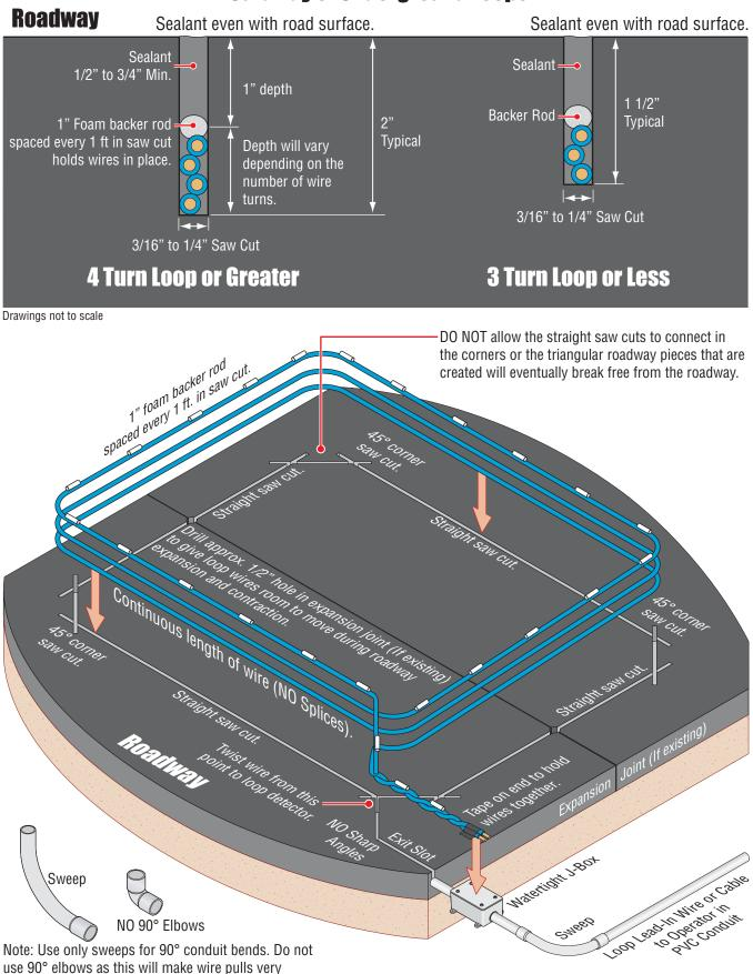
use 90° elbows as this will make wire pulls very difficult and can cause damage to wire insulation.
