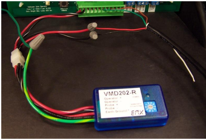
Typical connection to operator with VMD202 remote control installed.
