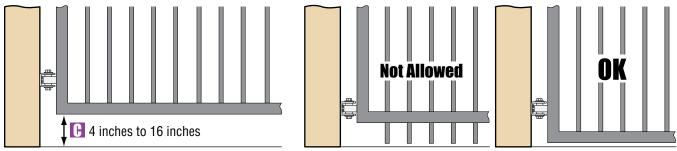
Gates shall have smooth bottom edges, with vertical bottom edged protrusions NOT exceeding 0.50 inches (1.2 cm).
