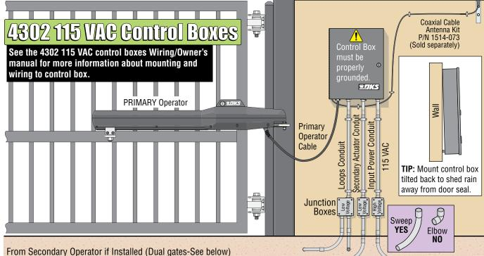
**Dual Gate Operators (115 VAC or Solar Control**
