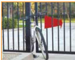
entrapment prevention system reverses gate on contact
