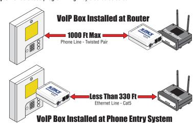
**Ethernet Line** Cat5 To Router DO NOT use this VoIP device to make 911 calls. to LAN **Phone Line** To Telephone Entry System PHONE IN (Twisted Pair) Plug 12 VDC
