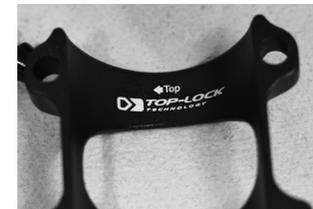
c. Double check the orientation of the stem faceplate by confirming which is the top on the reverse side.
