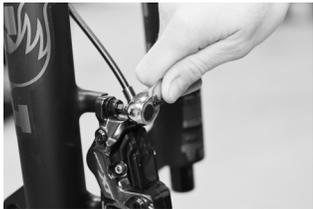
b. Using a 5mm, install the caliper to the fork. Tighten both bolts down evenly until snug, then back off each bolt half a rotation and leave loose for now.
