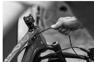
c. While gently pulling on the seatpost remote cable housing, continue to insert the seat post to your desired height.
