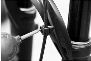
a. Attach the brake hydraulic line to the fork arch using the manufacturer's integrated clamp.
