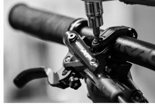
b. Using a 4mm Alley key, loosen the brake lever clamp bolts and adjust the location for your brake levers.
