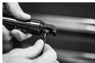
a. Fit cable end nut into the cradle at the bottom of the seatpost.
