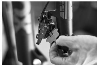
e. Remove the bike out of box, remove brake pad spacer from the caliper and keep the spacer for any future transportation where the wheel needs to be removed.
