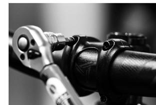
d. Using a 4mm Allen key, re-install faceplate and faceplate bolts adhering to the manufacturer's specifications.
