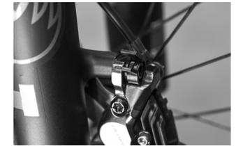
i. Install the nylon anti-rotation devices (in small parts box) on the brake bolt heads.
