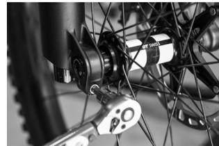
f. Insert front wheel into the dropouts. Using a 6mm Allen key for the Fox 36 fork, tighten the axle to 9Nm. Then tighten the pinch bolt under the axle head to 5Nm to lock the axle in place.
