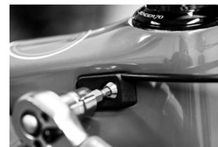
e. Using a 4mm Allen key, pull gently on remote cable housing and re-tighten cable port to 1-2Nm.
