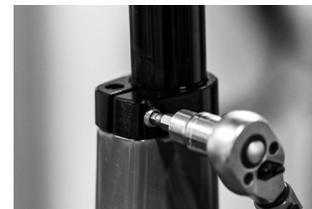
d. Tighten the seatpost clamp to 6Nm.
