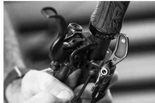
c. Using a 3mm Allen key, dial in the shifter and dropper remote position. They can be moved up and down/in and out to get the perfect placement.
