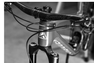
b. Ensure cables are properly routed and mount the handlebar on the stem.
