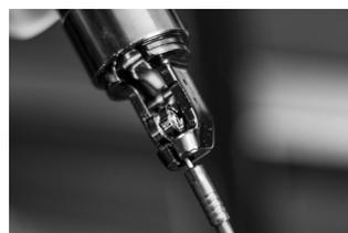
b. Pull the housing away from the cable end nut and align the housing into the housing stop at the bottom of the seatpost.
