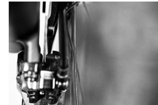
h. With the brake lever still applied, tighten the two caliper bolts. Once tight, release the brake lever and spin the front wheel to test any drag between the rotor and caliper. If the wheel is spinning freely without sound, using a 5mm Allen key, tighten the two caliper bolts to 8Nm.
