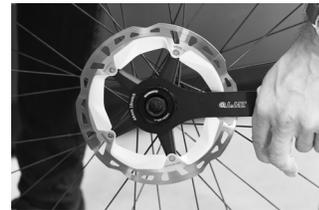
d. Insert rotor onto the hub and using a 44mm 16 notch installation tool, torque lock ring to 40Nm.
