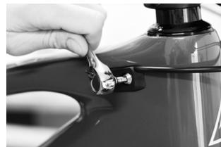
a. Using a 4mm Allen key, loosen the dropper post cable port (drive side, near the head tube) one full turn.
