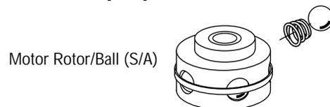
**Note:** If a separate motor race is not available, work a wide rubber band around the outside of the motor rotor to hold the ball pistons in their bores.
