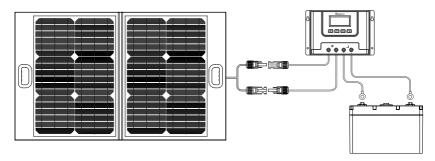
To expand the output power, please connect multiple E.FLEX 50 in parallel by joining the female and male Solar Panel Connectors of each E.FLEX 50 together with solar parallel branch connectors (not included).
