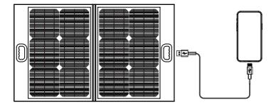
To charge handheld gaming consoles, DSLR cameras, or other USB-C enabled devices, please slide the Slide Switch to the left position and connect the device to the E.FLEX 50's USB-C Port using a USB-C charging cable (not included).
