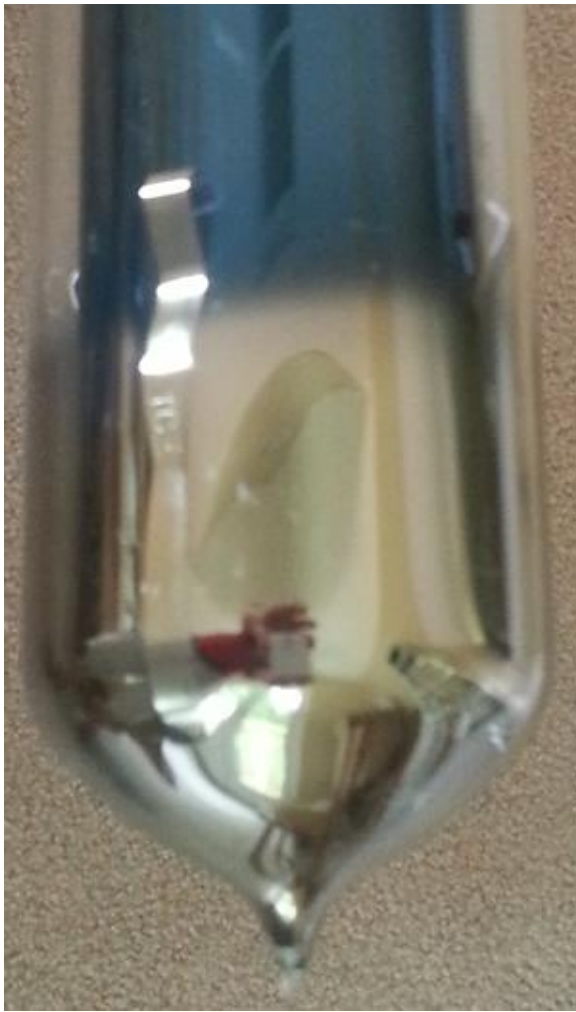
Good Tube with Metallic Bottom (Existing Vacuum)
