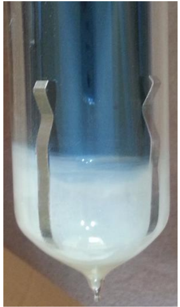
Bad Tube with White Bottom (Vacuum Lost)
