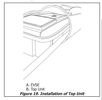
3. Install cord into top wiring chamber of the top unit.
