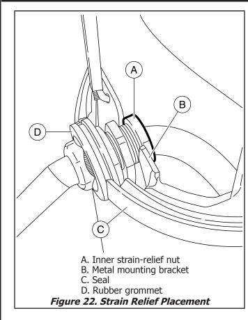
2. Tighten the inner strain-relief nut (A) inside the bollard hand tight. Using expandable pliers, tighten the nut an additional 1/4 turn.
