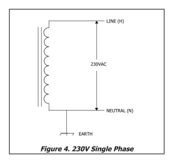
WARNING: The EVSE is a single-phase device. When connecting the line and neutral wires, take care that the service transformer secondary connection is known, and the wires from the main circuit breaker panel are correctly connected and labeled. The following service connections are primarily used in Europe and Australia (sometimes known as "TT Power Grid"). Please reference the following diagram. The line, neutral, and earth outputs on the illustration correspond to the inputs on the EVSE.
