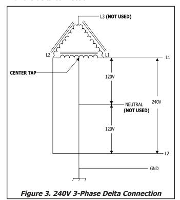
NOTE: The third line (L3 on the illustration of the delta) is 208V, with respect to the neutral, and is sometimes referred to as a "stinger."
