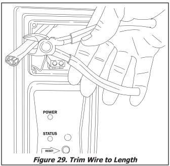
13. Trim the wire to a length sufficient to make the connections to the Charge Station terminal block.
