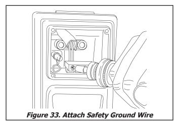
18. Attach safety ground wire through the slot on the ground terminal. Hand-tighten grounding lug.
