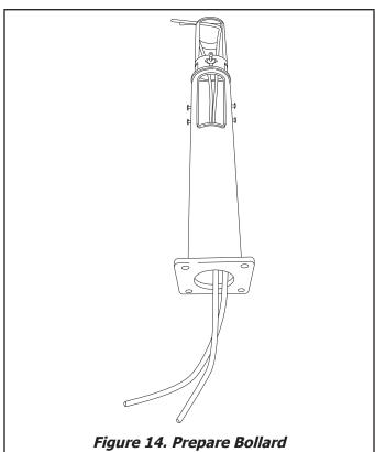
1. Feed the length of the charging cable through the exit hole in the side of the bollard.
