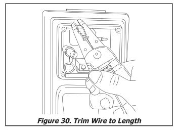
14. Strip back 1 1/4 in. (32 mm) of the wire jacket and 3/8 in. (10 mm) from the ends of the individual conductors.
