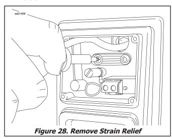
12. Remove the strain-relief assembly from the wiring chamber.
