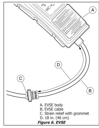
NOTE: The EVSE has been factory set at 30 amp output for a 40 amp circuit. Proceed to "Standard Installation" if installing on a 40 amp circuit. For all other amperages, complete Steps 2 and 3 for EVSE adjustment.
