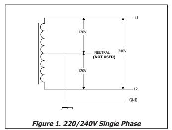
WARNING: The EVSE is a single-phase device. Do not connect all three phases of a 3-phase feed. Only three wires are connected, take care that the service transformer secondary connection is known, and the three wires from the main-panel circuit breaker are correctly connected and labeled.
