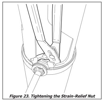
NOTE: Do not overtighten the strain-relief nut. The grommet may pull through.
