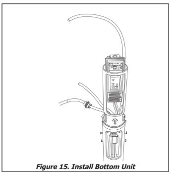
. Slide bottom unit into mounting position. Take caution not to scrape the front surface of the EVSE against the bollard. Cables and cords will pass by the sides of the EVSE.
