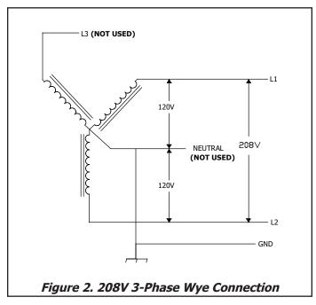
NOTE: A current-carrying neutral is not required for the EVSE for 208V connections.
