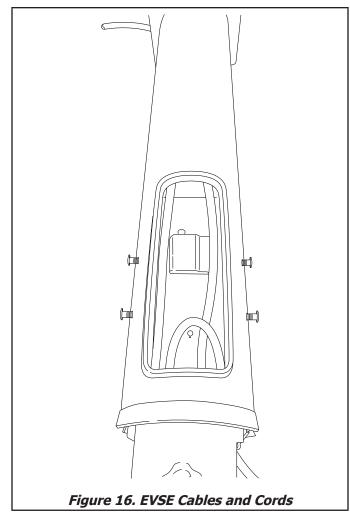
4. Install cord into top wiring chamber of the bottom unit.
