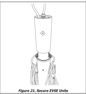
1. Position the strain relief at the bottom of the side slot metal mounting bracket in the steel bollard. Position such that the rubber grommet (D) seats on the opening of the lower plastic bollard cover. Repeat on opposite side.
