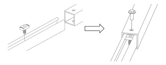
8. Attach tilt legs to lower saddle L-brackets. Adjust the tilt angle by adjusting the tilt arms and lower saddle to the desired angle of tilt then tighten the U-bolt/band clamp on the lower saddle. For 5/16" hardware tighten using 1/2" wrench to 10-12 ft-lb torque.
