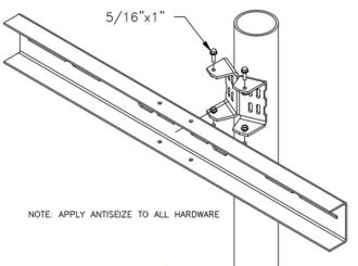
4. Loosely fasten the lower easy mount bracket to the pole. Use the below chart for rough spacing between the two saddles.
