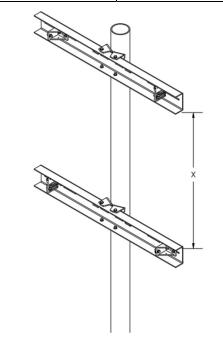
5. Lay rails on module holes (but do NOT attach) to determine angle bracket spacing (see image below). Measure between the inside of the module rails. Mount angle brackets to saddles using the 5/16" hardware provided. Tighten using 1/2" wrench to 10-12 ft-lb torque. Apply anti-seize.
