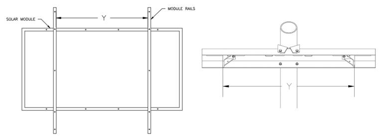
6. Attach panel rails to upper saddle L-brackets using 5/16" hardware provided. Apply anti-seize.
