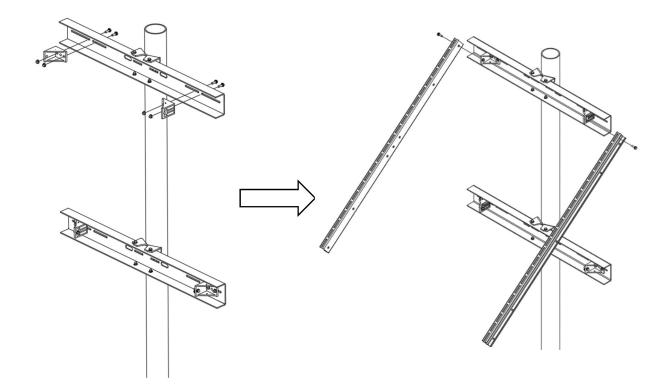
7. OPTIONAL: Drop spring nut into tilt leg strut and rotate to lock into place. Slide strut and spring nut into tilt leg tube and adjust to desired length. Longer legs, decrease tilt: shorter legs, increase tilt. Tighten 3/8" hardware using 9/16" wrench to 18-20 ft-lb torque.
