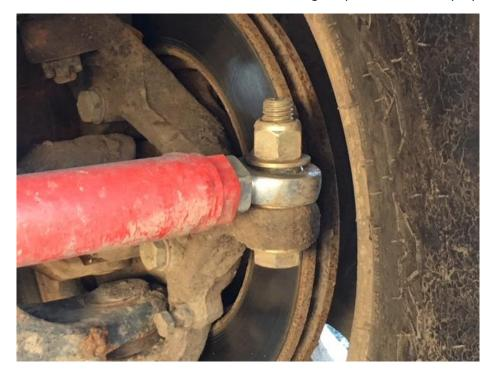
You then want to use the 5" bolt on the Passenger side knuckle using the picture below for proper order.
