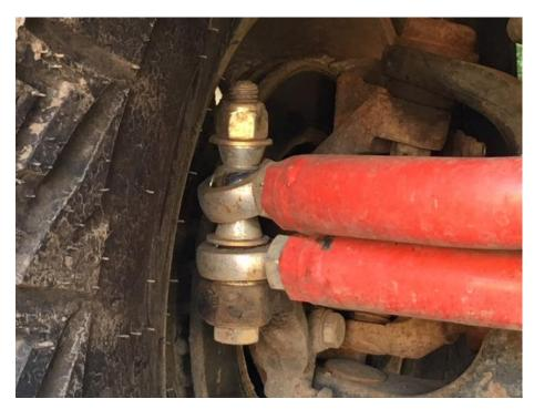
Now the final connection on the pitman arm, using the 4" bolt using the picture below for proper order.
