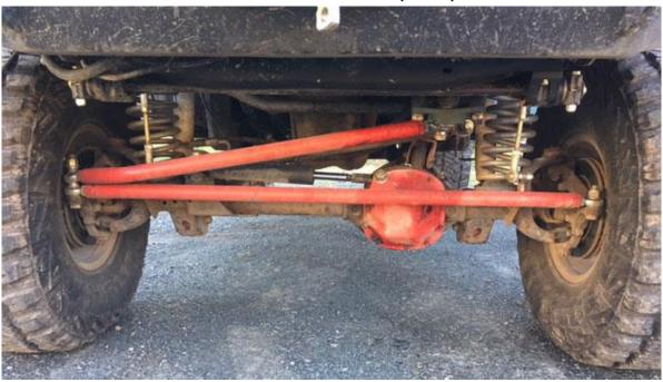
You will want to use the 3" bolt on the driver side, knuckle using the picture below for proper order.
