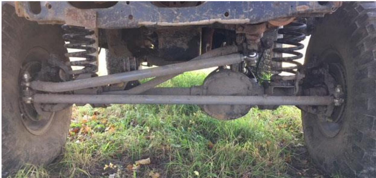
You will want to use the 3" bolt on the driver side, knuckle using the picture below for proper order.
