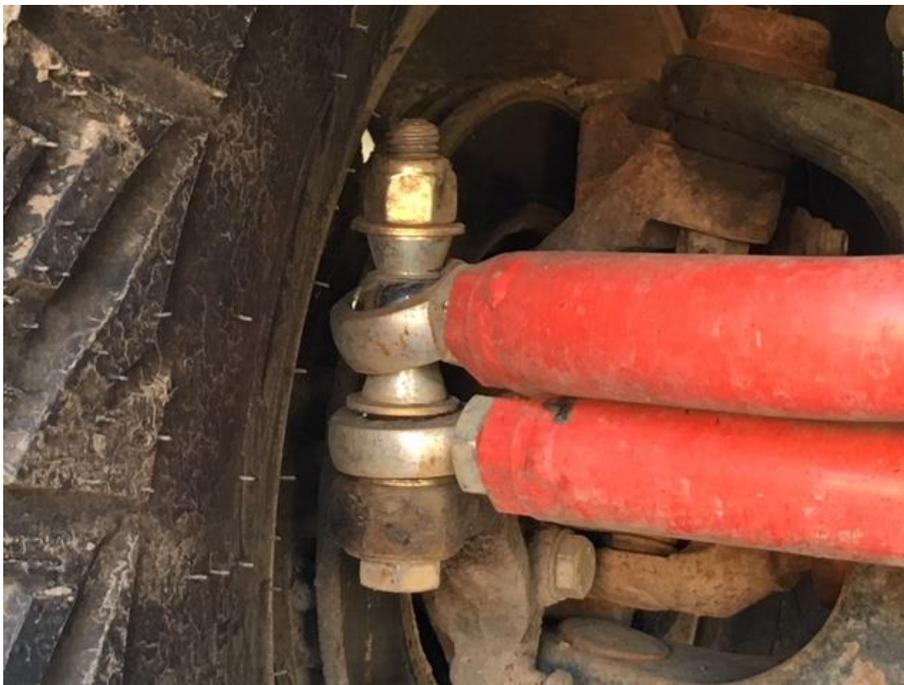
Now the final connection on the pitman arm, using the 4" bolt using the picture below for proper order.
