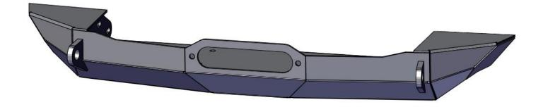
The Stump Winch DIY bumper kit is designed to be built with basic welding and metalworking skills and should take approximately 4-8 hours to complete.
