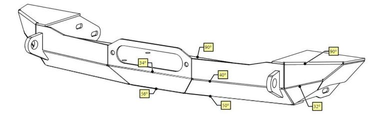
The weld brackets are tabbed and slotted onto the winch plate, bend the back lip to 90° and then weld the brackets to the winch plate.
